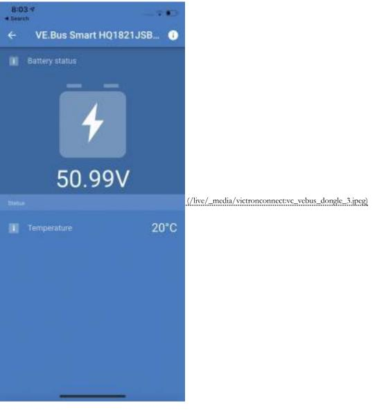
It takes a bit of time before a Multi is detected. When the dongle detects a Multi, VictonConnect will identify the Multi in the Device list. Shortly after updating the firmware in VictronConnect only the dongle will show up in the device list. If connected, a re-scan will reveal the Multi.
