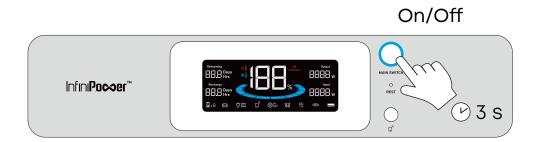
Press the main power button for 3 seconds to turn your power station on or off. When the "Battery Level" icon shows on the LCD screen, your power station is ready to charge devices.
