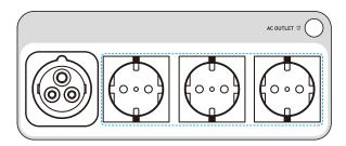
Press the AC outlet button and connect your devices to the TT-30R AC output port. The max output power via this port is 3,600W.
