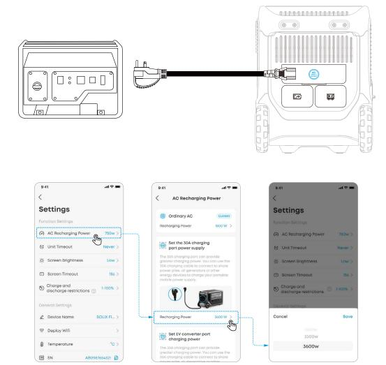
Turning off the generator directly may cause a power outage for several seconds. If you want to disconnect from Anker SOLIX F3000 Portable Power Station and the generator, please follow the steps below to avoid power disruptions.
