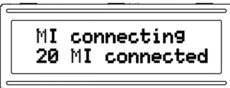
After the completion of network construction the EnverBridge start-up process finishes and EnverBridge is in normal monitoring working status. It will take a relatively long period of time before the monitoring interface information shows up on the LCD screen. EnverBridge will **unlock** and **construct the network** again automatically if there is a failure of network construction.
